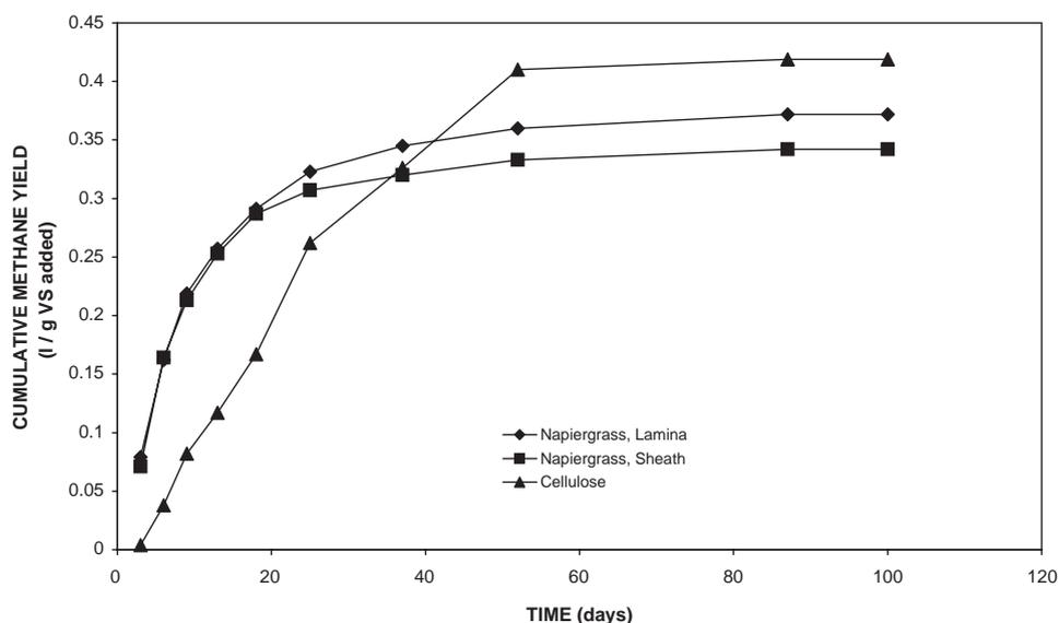
Fig. 2. BMP cumulative methane production of napiergrass and cellulose.
