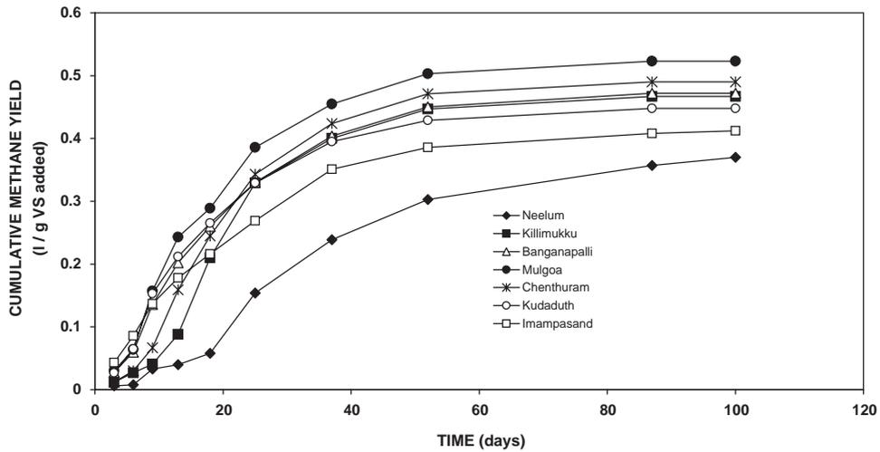
Fig. 3. BMP cumulative methane production of mango peel varieties.
