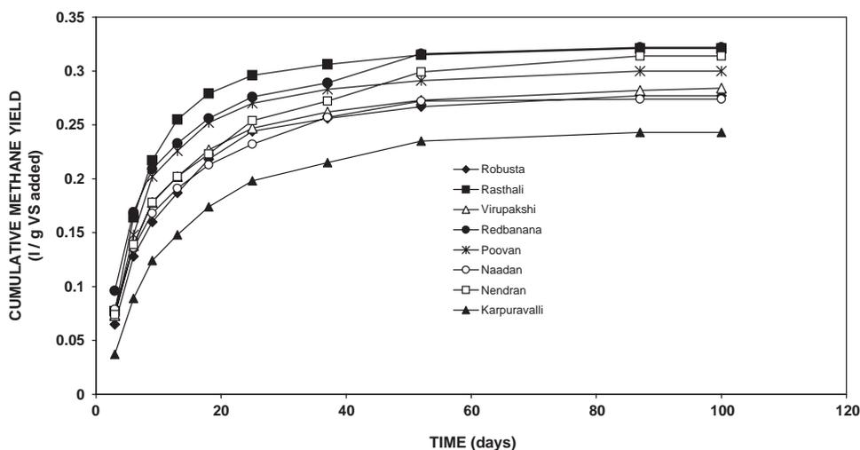
Fig. 4. BMP cumulative methane production of banana peel varieties.
